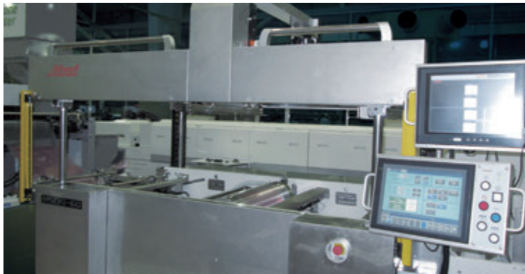
As the up and down movements of the screen frame are controlled by the servo motor, accurate digital clearance adjustments are possible.
