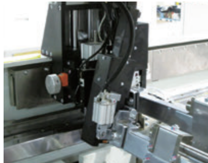
Squeeze pressure and flood bar drop-down are also controlled by a servo motor, and they are operated on the touch panel.
