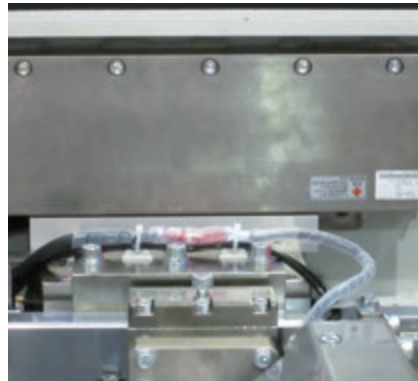
The screen frame is driven by the linear servo motor.
